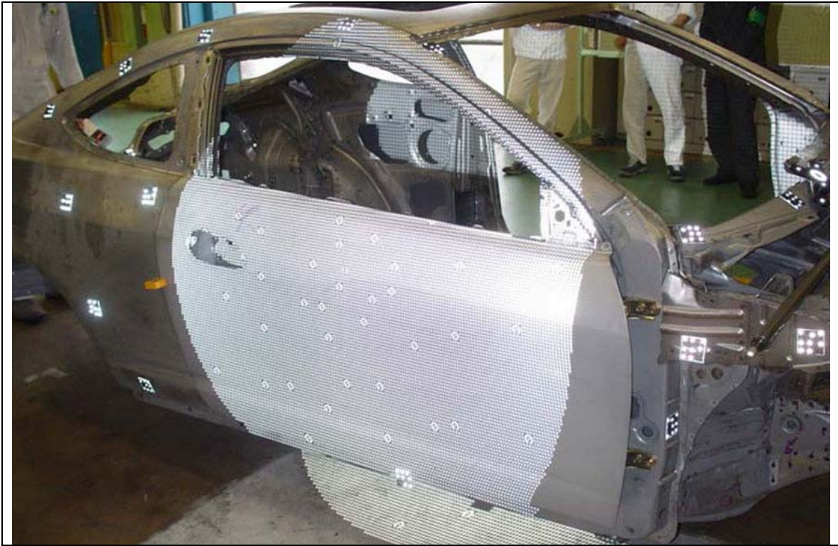
Typical surface measurement to verify door position
