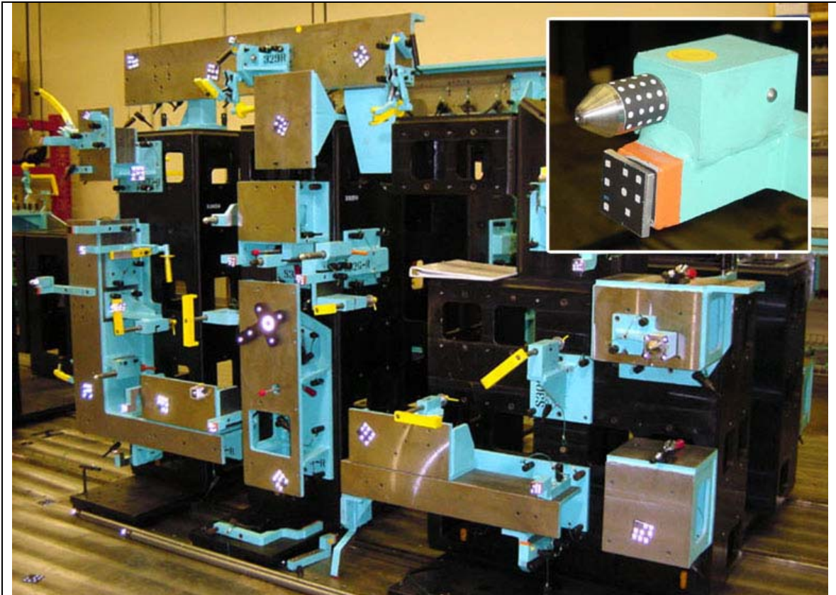
Typical fixture measurement carried out at Ford
