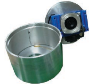
Figure 3. INCA3 and underwater canister
