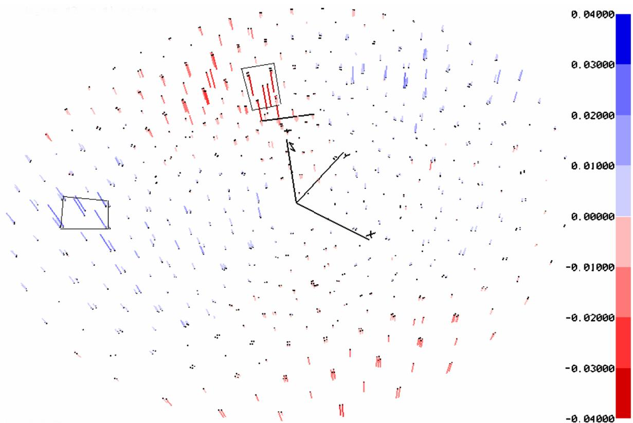
The differences are very systematic in nature. Only two panels appear to have moved. They are outlined above. They stand out as being significantly different from the surrounding points and from the first measurement. The tables below list the amount the points on the panels moved as well as the average movement.
