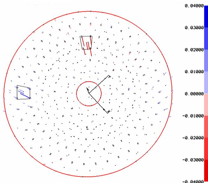
The differences are again very systematic in nature. The two panels that appear to have moved are outlined above. They stand out as being significantly different from the surrounding points and from the measurement before adjustment. The tables below list the amount the points on the panels moved as well as the average movement.
