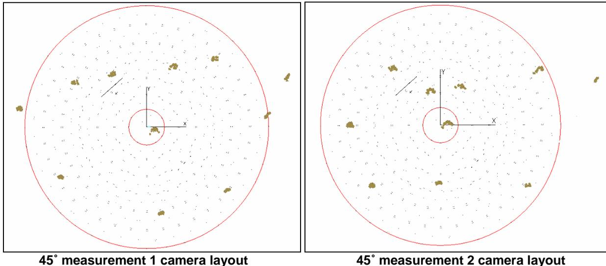
Notice not only how poor the camera geometry is for the second measurement compared to the first but also how much poorer the geometry is for both measurements than for the 90° measurement shown earlier. The cameras were only rarely positioned outside the edge of the antenna as desired. Nor are they well arranged at 45° spacing around the antenna. Although
