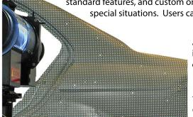
All targets are illuminated by a small, low-power flash system which provides consistent illumination whether taking pictures in low or high ambient light conditions varying from complete darkness to outside in full sunlight.
